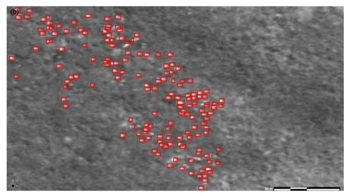
Fig. 2. The results of automated saiga counting on a satellite image using artificial intelligence: (a) - segmentation of the image and successive analysis of each segment for concentration of bright small-sized objects with shadows (stage 1 - DCNN-C), (b) - analysis of the image's fragments that have been classified by DCNN-C as "containing at least one saiga" (stage 2 - DCNN-I).
